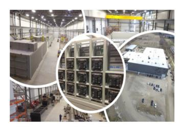
The core focus of the 100,000 square feet facility in Southern Ontario is the assembly of custom power distribution solutions. The plant is equipped with sheet metal fabrication, structural weld, powder paint booth, assembly and test area. Low voltage switchgear assemblies are built on
