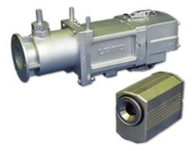
Using AMETEK Land's leading-edge infrared sensing to measure both furnace load and background temperature, the Furnace Thermometer System (FTS) links to the advanced Landmark Graphic signal processor for a true temperature of the reheat furnace load unaffected by reflections from a hotter background.
