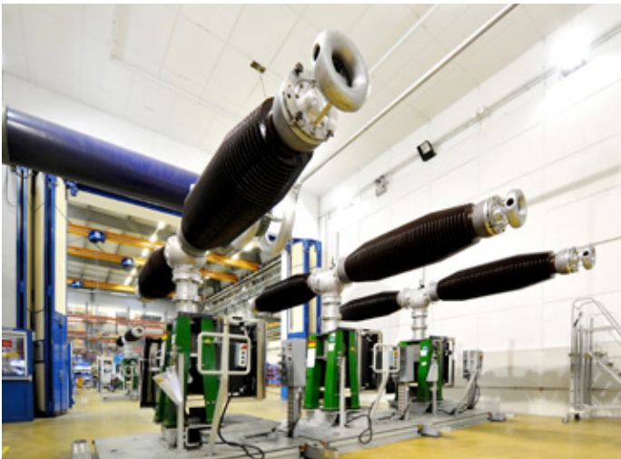
High Voltage Testing of Live Tank Circuit Breakers
