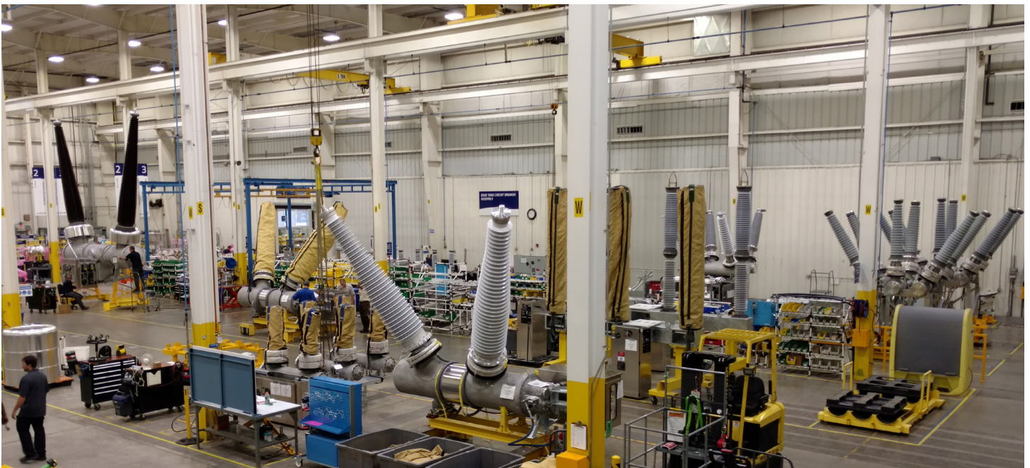
Clean room assembly hall - dead tank circuit breakers before routine testing.
