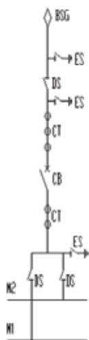
Busbar Coupling Bay Configuration
