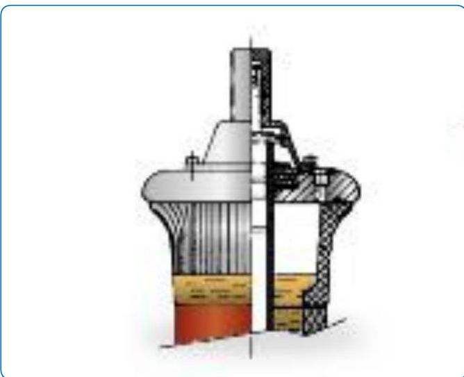
Fig. 2: Oil level indicator for prismatic glass and metal head
