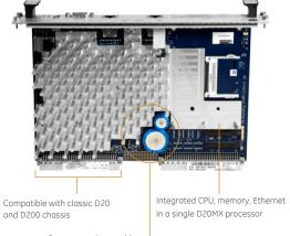
Super capacitor enables maintenance-free, battery-less operation
