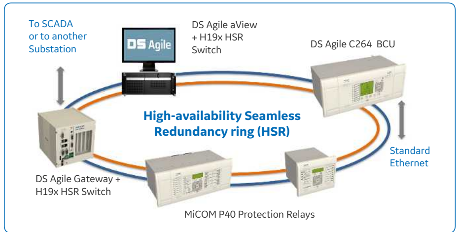
IEC 62439-3-5 HSR ring, Ethernet-based architecture
