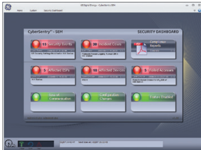
The CyberSentry SEM security dashboard displays alarm notifications in a single view, enabling operators to take quick action.
