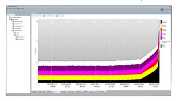
Displays the total dissolved combustible gas as relative concentrations within a trend chart. This view allows the user to quickly gauge the relative ratio concentrations of the individual gases.
