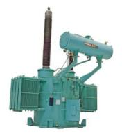
**Shunt reactors** are the most compact and cost efficient means of compensating capacitive generation in long transmission lines. They are placed permanently in service to stabilize power transmission, or switched in under light load conditions.
