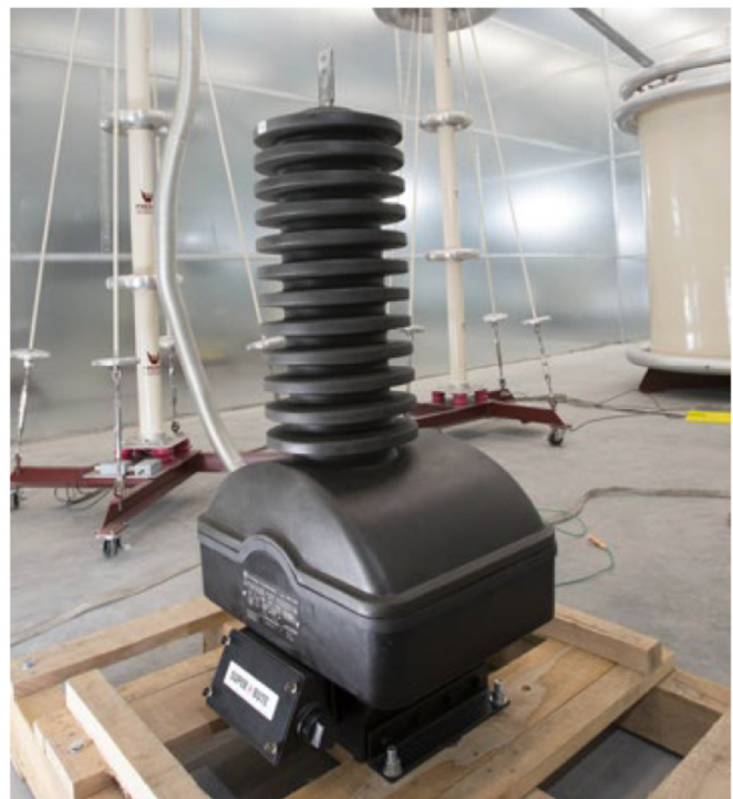
Impulse and partial discharge testing a 72.5 kV, 350 kV BIL substation-class PT. Both chop wave and full wave impulse testing is performed as a routine test on all SUPERBUTE units 8.7 kV and above
