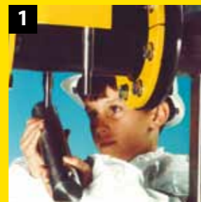
1 Remove tie rod pins and lower pinch bar
