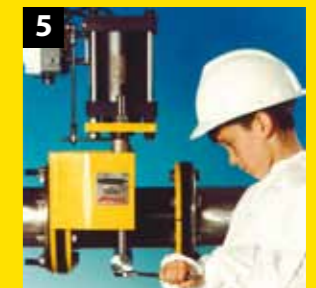
5 Replace lower pinch bar and tie rod pins
