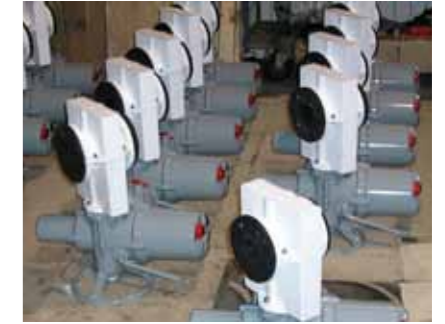
Gold Coast Desalination Lime Dosing Valves
