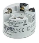
Output loop-powered head transmitter for transmitting RTD and TC sensor signals as well as resistance-type sensor and voltage sensor signals via HART(R) communication or 4 ... 20 mA, freely configurable, screw connection.
