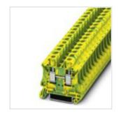
Ground modular terminal block, connection method: Screw connection, number of connections: 2, cross section: 0.2 mm<sup>2</sup> - 10 mm<sup>2</sup>, AWG: 24 - 8, width: 8.2 mm, height: 46.9 mm, color: green-yellow, mounting type: NS 35/7,5, NS 35/15
