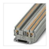
Feed-through terminal block, nom. voltage: 800 V, nominal current: 24 A, connection method: Push-in connection, number of connections: 3, cross section:  $0.14~\text{mm}^2$  -  $4~\text{mm}^2$ , AWG: 26 - 12, width: 5.2 mm, height: 35.2 mm, color: gray, mounting type: NS 35/7,5, NS 35/15
