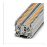
Feed-through terminal block, nom. voltage: 1000 V, nominal current: 41 A, connection method: Push-in connection, number of connections: 2, number of positions: 1, cross section: 0.5 mm² - 10 mm², AWG: 20 - 8, width: 8.2 mm, height: 42.2 mm, color: gray, mounting type: NS 35/7,5, NS 35/15
