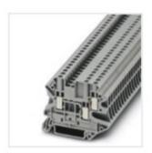
Feed-through terminal block, nom. voltage: 500 V, nominal current: 24 A, connection method: Screw connection, number of connections: 3, cross section: 0.14 mm<sup>2</sup> - 4 mm<sup>2</sup>, AWG: 26 - 12, width: 5.2 mm, height: 46.9 mm, color: gray, mounting type: NS 35/7,5, NS 35/15
