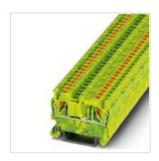
Ground modular terminal block, connection method: Push-in connection, number of connections: 2, cross section: 0.14 mm<sup>2</sup> - 4 mm<sup>2</sup>, AWG: 26 - 12, width: 5.2 mm, height: 35.3 mm, color: green-yellow, mounting type: NS 35/7,5, NS 35/15
