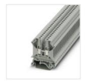
Feed-through terminal block, nom. voltage: 800 V, nominal current: 32 A, connection method: Screw connection, number of connections: 2, cross section: 0.2 mm<sup>2</sup> - 6 mm<sup>2</sup>, AWG: 24 - 10, width: 6.2 mm, color: gray, mounting type: NS 35/7,5, NS 35/15, NS 32
