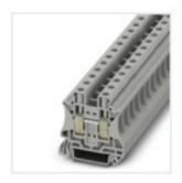
Feed-through terminal block, nom. voltage: 1000 V, nominal current: 57 A, connection method: Screw connection, number of connections: 2, cross section: 0.5 mm<sup>2</sup> - 16 mm<sup>2</sup>, AWG: 20 - 6, width: 10.2 mm, height: 46.9 mm, color: gray, mounting type: NS 35/7,5, NS 35/15
