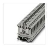
Feed-through terminal block, nom. voltage: 800 V, nominal current: 57 A, connection method: Screw connection, number of connections: 2, cross section: 0.5 mm<sup>2</sup> - 16 mm<sup>2</sup>, AWG: 20 - 6, width: 10.2 mm, color: gray, mounting type: NS 35/7,5, NS 35/15, NS 32
