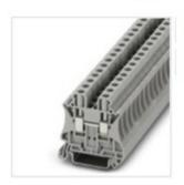
Feed-through terminal block, nom. voltage: 1000 V, nominal current: 41 A, connection method: Screw connection, number of connections: 2, cross section: 0.2 mm<sup>2</sup> - 10 mm<sup>2</sup>, AWG: 24 - 8, width: 8.2 mm, height: 46.9 mm, color: gray, mounting type: NS 35/7,5, NS 35/15
