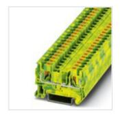
Ground modular terminal block, connection method: Push-in connection, number of connections: 2, cross section: 0.2 mm<sup>2</sup> - 6 mm<sup>2</sup>, AWG: 24 - 10, width: 6.2 mm, height: 35.3 mm, color: green-yellow, mounting type: NS 35/7,5, NS 35/15
