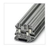
Feed-through terminal block, nom. voltage: 500 V, nominal current: 32 A, connection method: Screw connection, number of connections: 3, cross section: 0.14 mm² - 6 mm², AWG: 26 - 10, width: 6.2 mm, height: 46.9 mm, color: gray, mounting type: NS 35/7,5, NS 35/15
