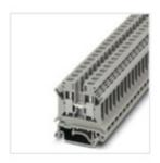
Feed-through terminal block, nom. voltage: 800 V, nominal current: 41 A, connection method: Screw connection, number of connections: 2, cross section: 0.2 mm<sup>2</sup> - 10 mm<sup>2</sup>, AWG: 24 - 8, width: 8.2 mm, color: gray, mounting type: NS 35/7,5, NS 35/15, NS 32
