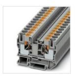
Feed-through terminal block, nom. voltage: 1000 V, nominal current: 57 A, connection method: Push-in connection, number of connections: 2, cross section:  $0.5 \text{ mm}^2 - 16 \text{ mm}^2$ , AWG: 20 - 6, width: 10.2 mm, height: 49.5 mm, color: gray, mounting type: NS 35/7,5, NS 35/15
