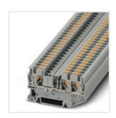
Feed-through terminal block, nom. voltage: 800 V, nominal current: 32 A, connection method: Push-in connection, number of connections: 3, cross section:  $0.2 \text{ mm}^2$  - 6 mm², AWG: 24 - 10, width: 6.2 mm, color: gray, mounting type: NS 35/7,5, NS 35/15
