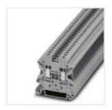
Feed-through terminal block, nom. voltage: 1000 V, nominal current: 24 A, connection method: Screw connection, number of connections: 2, cross section: 0.14 mm<sup>2</sup> - 4 mm<sup>2</sup>, AWG: 26 - 12, width: 5.2 mm, height: 46.9 mm, color: gray, mounting type: NS 35/7,5, NS 35/15
