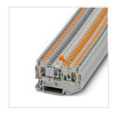
Knife disconnect terminal block, nom. voltage: 400 V, nominal current: 20 A, connection method: Push-in connection, cross section: 0.14 mm² - 4 mm², AWG: 26 - 12, length: 62 mm, width: 5.2 mm, color: gray, mounting: NS 35/7,5, NS 35/15
