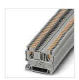
Feed-through terminal block, nom. voltage: 800 V, nominal current: 24 A, connection method: Push-in connection, number of connections: 2, number of positions: 1, cross section: 0.14 mm² - 4 mm², AWG: 26 - 12, width: 5.2 mm, height: 35.3 mm, color: gray, mounting type: NS 35/7,5, NS 35/15
