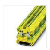
Ground modular terminal block, connection method: Screw connection, number of connections: 2, cross section: 0.14 mm<sup>2</sup> - 6 mm<sup>2</sup>, AWG: 26 - 10, width: 6.2 mm, height: 46.9 mm, color: green-yellow, mounting type: NS 35/7,5, NS 35/15
