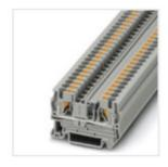
Feed-through terminal block, nom. voltage: 800 V, nominal current: 32 A, connection method: Push-in connection, number of connections: 2, cross section: 0.2 mm<sup>2</sup> - 6 mm<sup>2</sup>, AWG: 24 - 10, width: 6.2 mm, height: 35.3 mm, color: gray, mounting type: NS 35/7,5, NS 35/15
