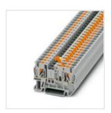
Knife disconnect terminal block, nom. voltage: 500 V, nominal current: 20 A, connection method: Push-in connection, cross section: 0.2 mm² - 6 mm², AWG: 24 - 10, length: 56 mm, width: 6.2 mm, color: gray, mounting: NS 35/7,5, NS 35/15
