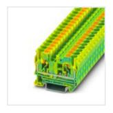
Ground modular terminal block, connection method: Push-in connection, number of connections: 2, number of positions: 1, cross section: 0.5 mm<sup>2</sup> - 10 mm<sup>2</sup>, AWG: 20 - 8, width: 8.2 mm, height: 42.2 mm, color: green-yellow, mounting type: NS 35/7,5, NS 35/15
