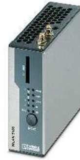
WLAN access point / client 2.4 GHz / 5 GHz
