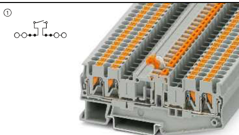
16 A, knife disconnect terminal block, 4 connections, 4 function shafts
