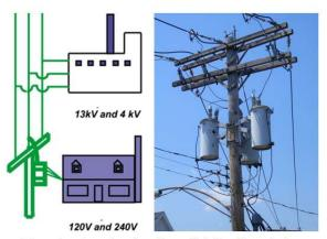
The Ontario electricity grid is made up of transmission lines crossing the province delivering electricity from generators to cities and communities. Generator produce the electricity we use. These facilities include water, wind, solar and natural gas. Local utilities own and operate the distribution system that delivers the power to homes and local businesses.
