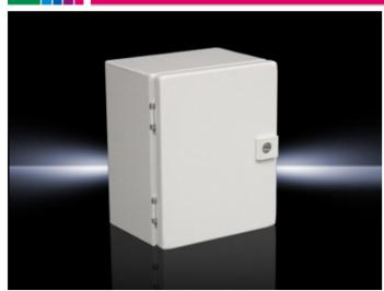
The JB enclosure offers protection for dense wiring and sensitive small instruments. These hinged cover junction boxes combine the advantages of the AE and KL series at an economical cost. Features include 180 degree hinge and slotted insert quarter turn latch. Foamed-in-place gasket and a knife-edge perimeter add extra protection.
