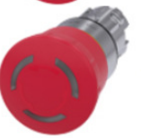
> 3SU10511HB200AA0 | 3SU10511HB200AA0 EMERGENCY STOP mushroom pushbutton, illuminable, 22 mm, round, metal, shiny, red, 40 mm, positive latching, acc. to EN ISO 13850, rotate-to-unlatch
