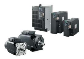
The SINAMICS V70 servo converter is primarily designed for controlling standard applications of turning and milling machines. It enables precision and efficiency of the machines through bus communication with the CNC control 808D ADVANCED, 3-fold overload capability and the 20-bit absolute encoder with high resolution in the feed motors SIMOTICS S-1FL6 and the main spindle motors SIMOTICS M-1PH1. Together, the products result in optimally matched axis packages.
