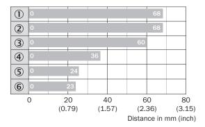
Max. sensing range  $S_n$ , flush or non-flush installation, non-magnetizable material
