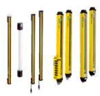
Multiple light beam safety devices are electro-sensitive protective devices with two or more light beams. If one or more of the light beams is interrupted, a deactivation signal is sent to the machine so that any dangerous state on a machine or system can be stopped. A system consists of a sender and a receiver. In active/passive systems, the sender and receiver are located in a housing unit while a deflection unit on the passive side provides beam deflection.
