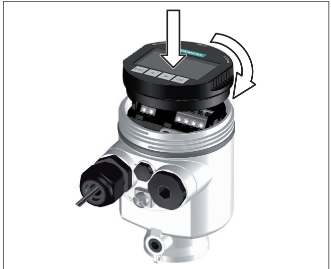
Fig. 22: Installing the display and adjustment module in the electronics compartment of the single chamber housing
