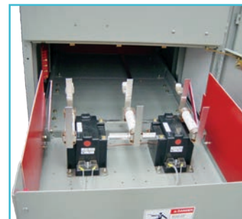
Figure 15: Type GM-SG non-arc-resistant, showing VT rollout tray withdrawn to allow inspection of fuses
