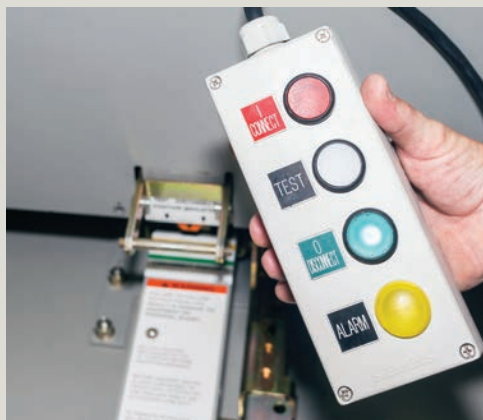
Figure 25: SIERS hand-held control pendant
