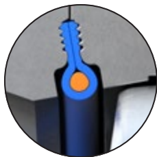
Disc in Open Position. Seat non-compressed.
