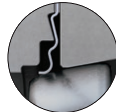
Disc in Closed Position. No line pressure.
