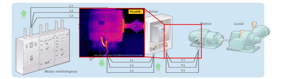
• Thermal imagers can be used to scan the motor drive output to identify hot spots or abnormal heating conditions.
