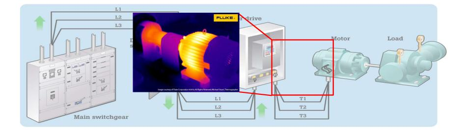
• Use a thermal imager to scan the component and look for irregular and non-uniform thermal patterns or anomalies.
