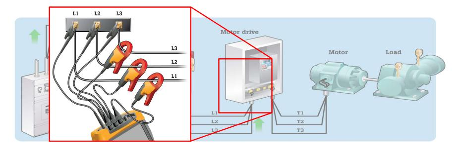
• Use a 3-phase power quality and motor analyzer to test power quality, electrical load and mechanical load.
