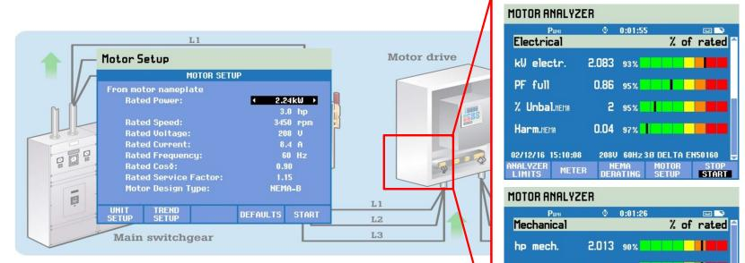
· Compare the motor electrical and mechanical parameters to the motor's nameplate.
