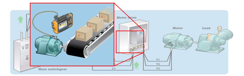
• Use the Fluke 810 vibration tester to measure looseness.
