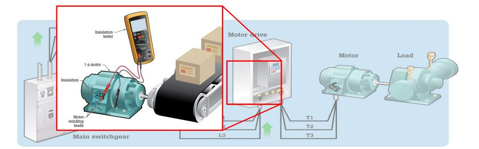
• Use an insulation resistance tester to measure each phase of the motor stator windings to ground.
