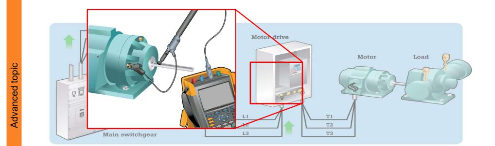
• Use an oscilloscope and carbon brush or stranded wire probe to measure the voltage between the motor chassis ground and the drive shaft.
