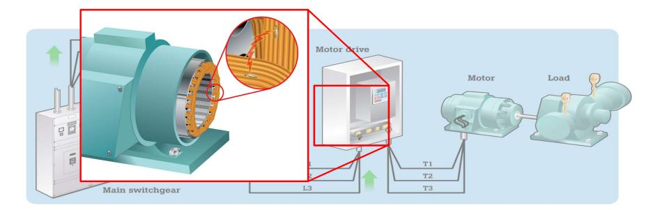
• Occurs when the insulation between motor windings deteriorates, causing a short circuit in the windings.
