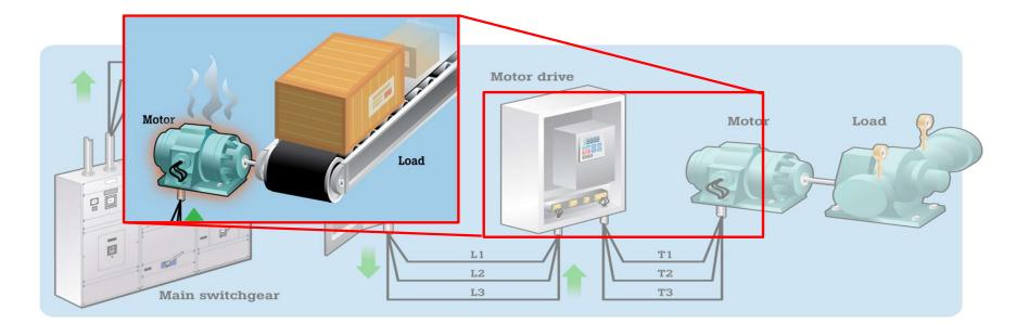
• The condition of the electrical feed can impact the performance of a motor and therefore negatively impact motor electrical and mechanical load factor.
