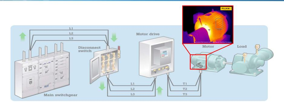
• Use either a thermal imager to look for abnormal heating or IR thermometer to compare suspect bearing to a known good bearing.
