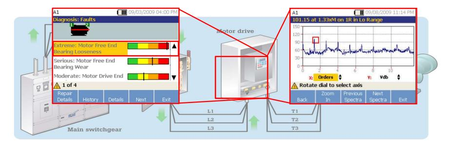
• The Fluke 810 does the interpretation for you using its extensive database of vibration profiles.
