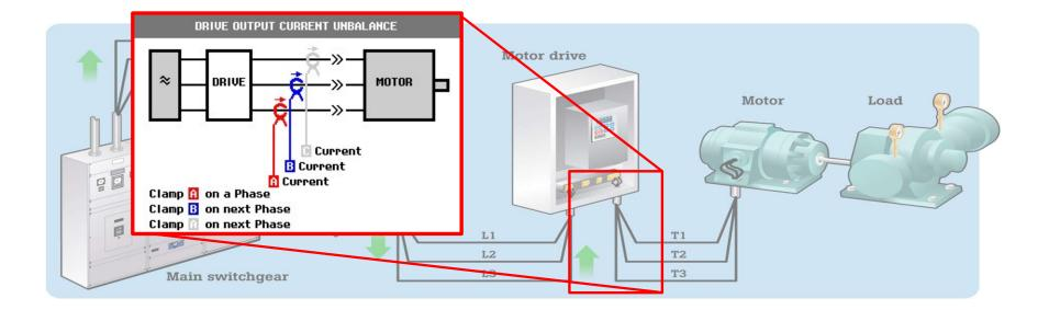
Use a dedicated motor drive analyzer with a current clamp on all three drive output terminals separately to measure the current draw on each terminal.
