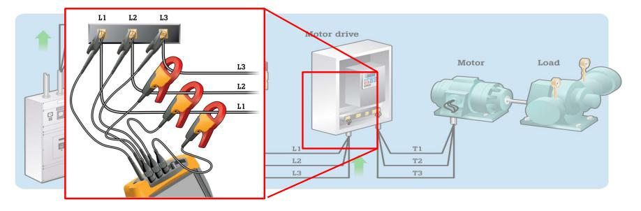
• Use a 3-phase power quality and motor analyzer to test power quality and measure electrical and mechanical load.
